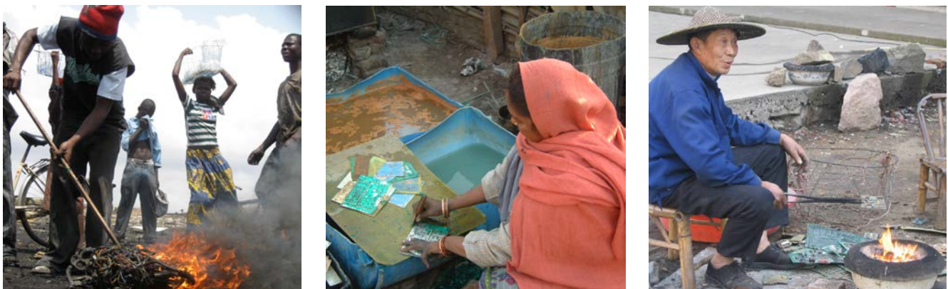
Figure 1: Typical recycling processes applied in the informal sector of developing countries (open burning of cables, leaching of gold from PWB, desoldering of PWB)
